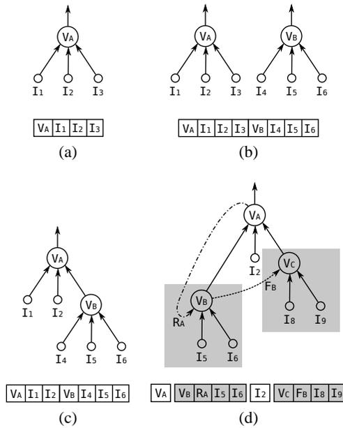
**Figure 1: Different examples illustrating CGE: (a) a simple three input network, (b) two subnetworks in parallel, (c) two subnetworks in cascade, (d) two subnetworks connected to a main network, including forward and recurrent jumper connections. Each example includes a neural network representation, and the corresponding CGE genome representation. All vertex genes in the genome representations possess a “number of inputs” attribute  $d_{in} = 3$ .**
