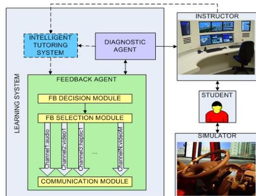
**Figure 2: Architecture of the feedback system where dashed lines represent optional components.**
