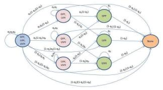
Figure 1: Markov chain for a UHF station.
