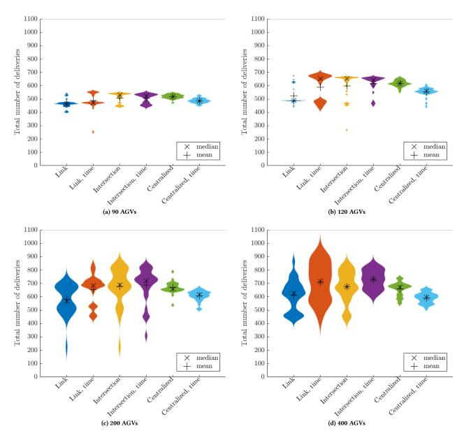
Figure 6: Violin plots of the team performance distributions at the end of 500 training epochs. The '+' symbol represents the mean and the '×' represents the median. All four multiagent team structures produce much wider distributions. Significant skew is observed at lower AGV numbers, whereas at higher AGV numbers the distributions become more symmetrical.
