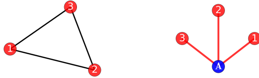
(a) Visibility graph. There must be common point from which 1 and 2 are visible. Similar is the case with (1,3) and (2,3). (b) There might exist a common coverage point from which all three strategic points are visible.
