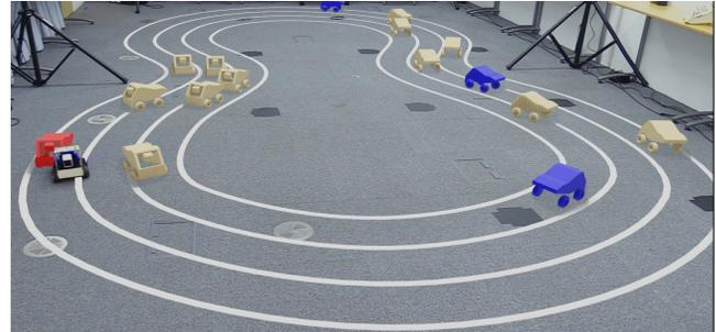
**Figure 1: Mixed reality multi-vehicle multi-lane traffic circuit including one real DeepRacer robot and 16 virtual ones.**
