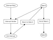
Figure 4: Interrupt implementation with Petri Net.
