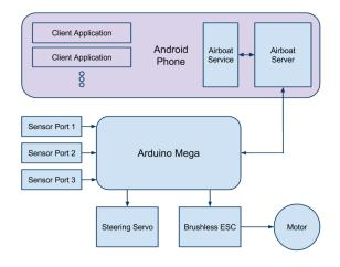
Figure 3: CRW system architecture
