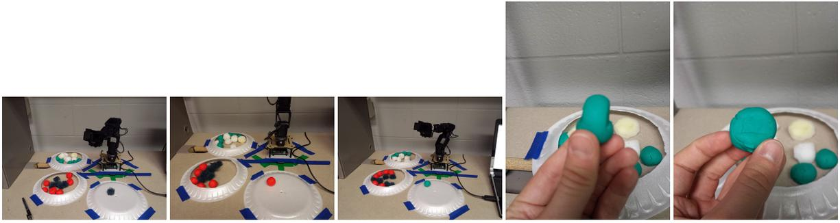
**Figure 4:** A series of snapshots of the Phantom Pincher arm sorting the balls. We introduce balls one at a time due to lack of sufficient space for several balls and the arm being small. The two bins with balls are visible on the left side of the arm. We show the deformed clay ball due to mishandling and the non-deformed clay ball on the right.
