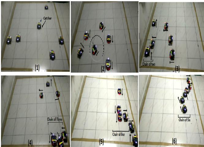
Figure 1: Robot simulation of Chain game with chains Tagging method and Escapees moving with K circle strategy. (1) Initial condition. (2) K circle around Catcher. (3) First Catch (4) Chain of three (5) Chain of five. (6) Chain completion
