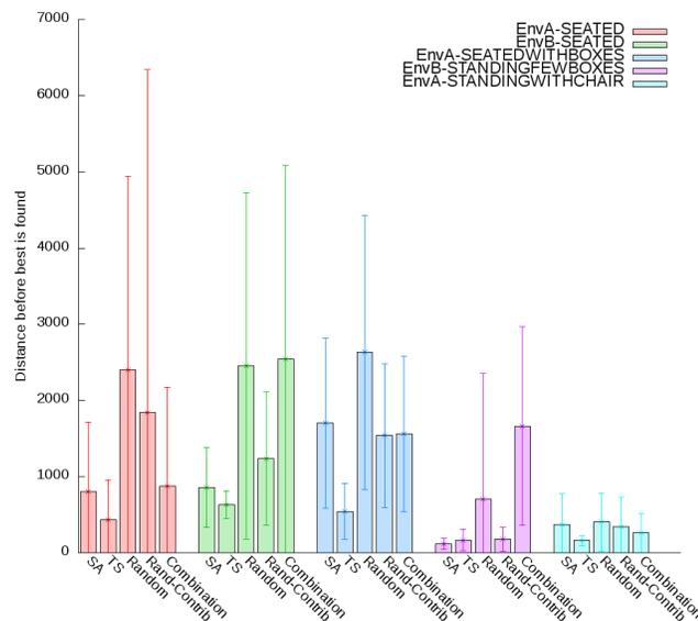
**Figure 6: Mean distance (meter) and standard deviation travelled by the robots before finding the best possible joint quality for the first time (50 experiments).**
