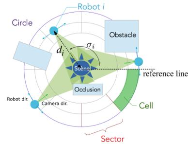
**Figure 1: Joint observation (coverage) of a scene (human activity) with a fleet of  $m = 3$  robots. The navigation model is based on circles with a spatial discretization in cells ( $C = 2$  circles and  $D = 8$  sectors).**
