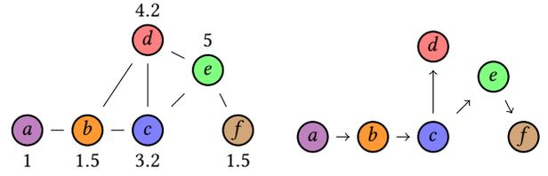
**Figure 4: (Left): the neighborhood graph in Example 1. The numbers represent utilities. (Right): a communication tree in convergence. In this case, agent 'a' is  $i_{\min}$  and therefore the root of the tree.**
