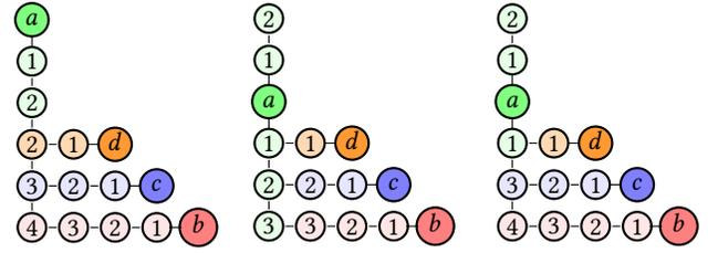
**Figure 5: A pathological non-convex discrete example. Different from grid spaces, nodes are connected by edges. Left: Voronoi partition. Middle: A move of agent  $a$  changes partitions outside of the neighborhood. Right: Changes in  $\mathcal{P}$  are confined inside the neighborhood.**
