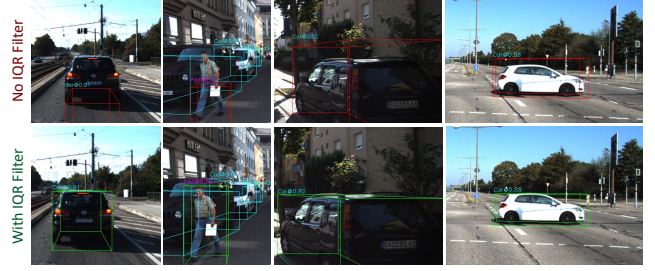
Figure 4: Effect of IQR filtering on 3D box reconstruction. Top row shows boxes reconstructed without IQR filtering. Bottom row shows results after filtering. In the first two examples (from left), low outlier returns within the same footprint shift the estimated bottom plane downward, leading to excessive height and activation of the default height constraint, which reduces 3D IoU. IQR removes these low outliers and restores a correct bottom estimate. In the third and fourth examples, the bottom plane is correct but a few high outliers inflate the top estimate. After IQR filtering, the top plane aligns with the vehicle roof, resulting in a tighter and more accurate 3D box.
