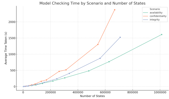
Figure 6: Runtime of symbolic model checker for different attacker goals as number of states increases.
