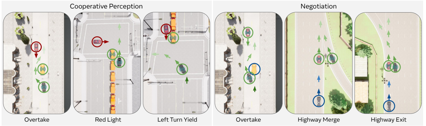
Figure 3: Overview of Scenarios and Agent Roles. Green circles: Focal agents, agents aim at establishing coordination through communication; Red circles: Potential colliders; Blue circles: Background agents.
