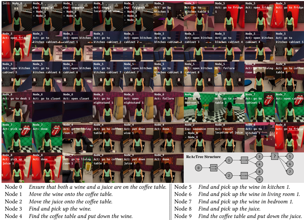
Figure 3: Success case of ReAcTree on the WAH-NL dataset using Qwen 2.5 72B. The snapshot of each step and the tree structure of nodes are shown. The subgoal of each node is also listed.
