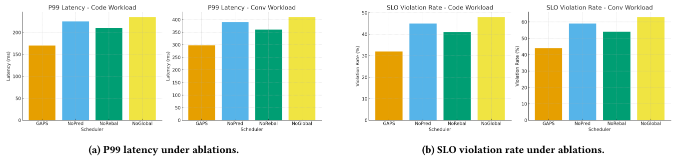
Figure 4: Ablation study on code and conversational workloads. Removing prediction, rebalancing, or global awareness significantly degrades performance compared to full GAPS.
